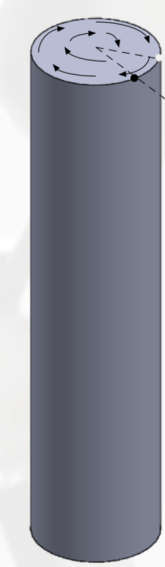
Figure 6: Loading conditions used to obtain G_{12} .
