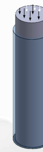
Figure 4: Loading conditions used to obtain the longitudinal modulus of the effective fiber.
